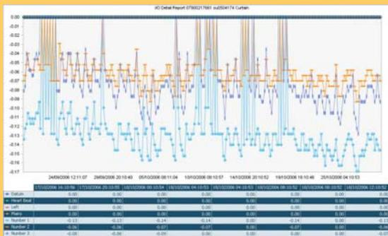
The intermediate phase is data cleansing and removal of 'odd' data. The 'lost signal' values and the wide range over a short period. Below we have plotted the outcome using trendline analysis.
