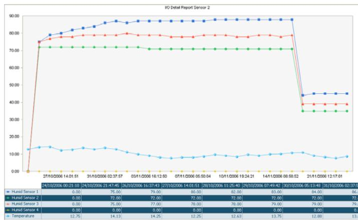
The system hadn't been calibrated on installation but using data from the neutron probe we were able to re-set the values from the offices here in the Midlands rather than have to drive a round trip of 200 odd miles to visit site, dig them up and re-code. Another major advantage.
