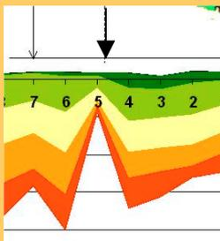
Incidentally, the anomaly at Station 6 coincides with NP3 where gravel was encountered and we suspect they are influencing the readings to the right - Stations 14, 15 ...
